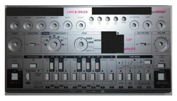
The PCB allows for installing a second row of sockets over the existing one (you need to scrape off a bit of the plastic spacer over the filter input socket if you want to have a socket there too, but the rest is easy). Installing 3.5 mini jacks (Tayda) vertically is okay if you bend the solder lugs. Common sub miniature switches also fit if you bend their legs.
