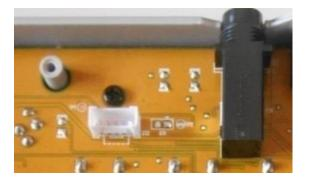
**Gate Input** (adapted from xoxbox wiki): Tip lug of input jack socket goes to 22k resistor. The other end of 22k resistor goes to a diode, the cathode of which goes to base of T30. The junction between T30 and R142 goes to a solder point on the **back of the PCB**. This only works when physical ground is connected (i.e. output/usb cable plugged or ring lug of your CV input socket connected to TP1 or Pin5 of X12).
